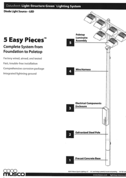
Schematic of Lighting Pole
