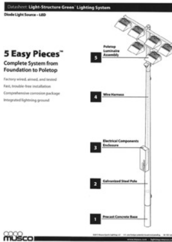
Schematic of Lighting Pole
