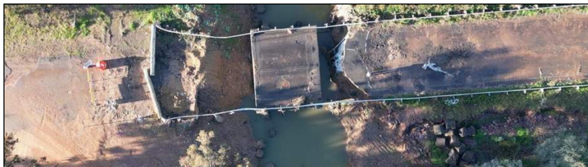
Figure 2 Existing Bridge Aerial View - approaches washed away.
