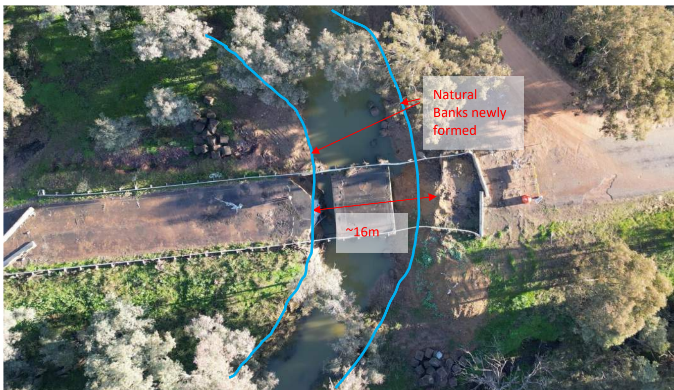
Figure 13 Natural Bank Lines and apparent 16m span
