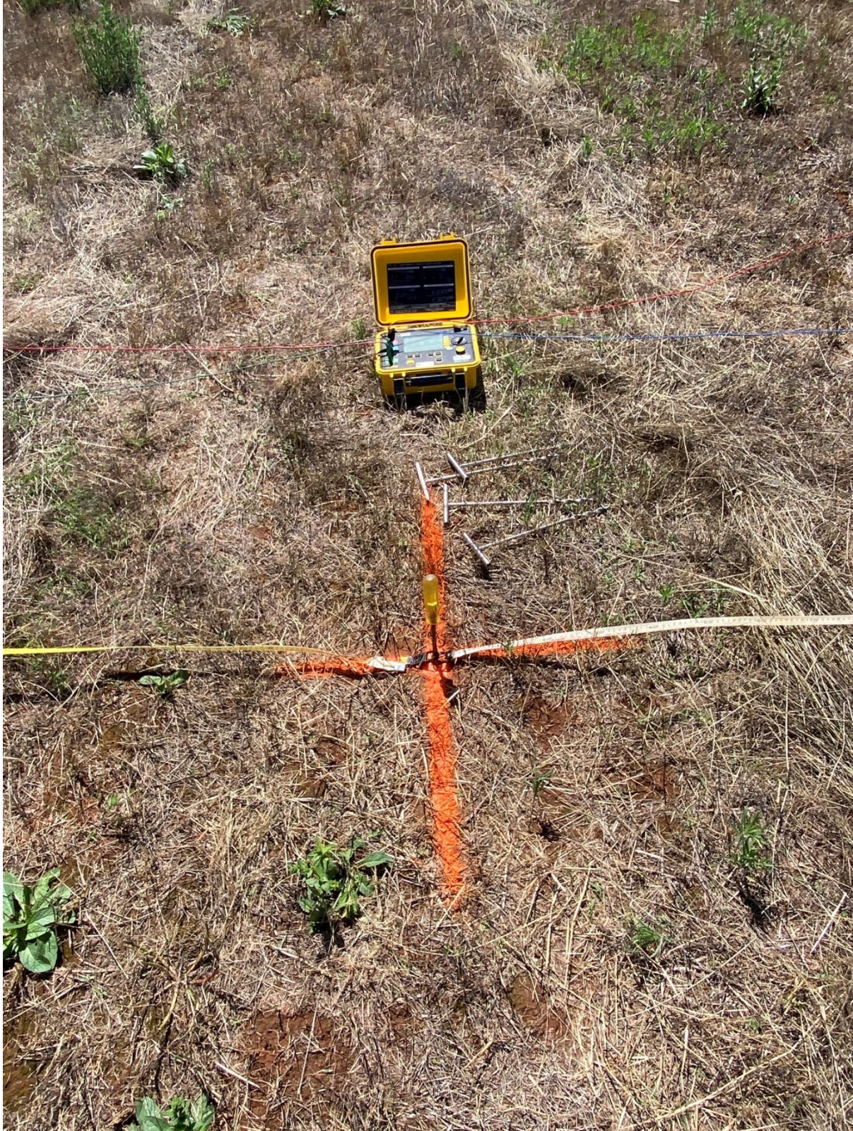
Photograph 7: General arrangement of field electrical resistivity testing.
