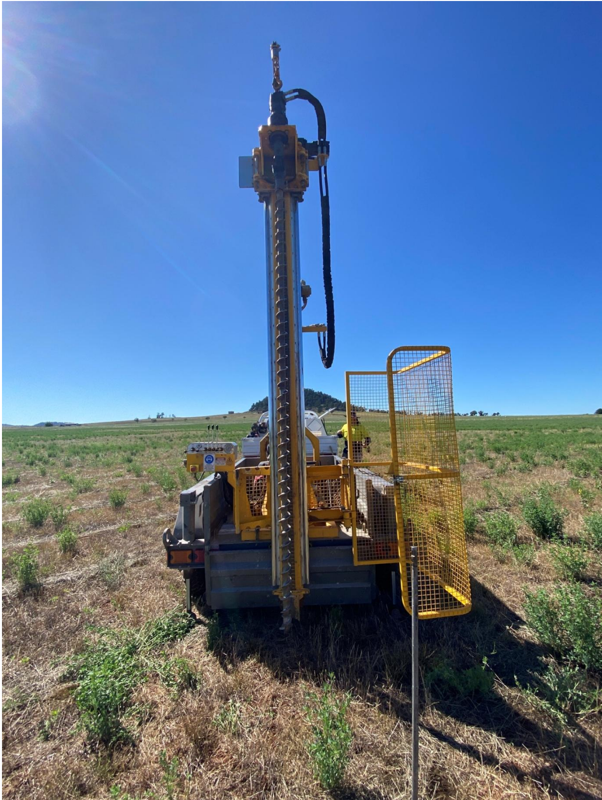
Photograph 5: The sampling method used on site – Power auger.
