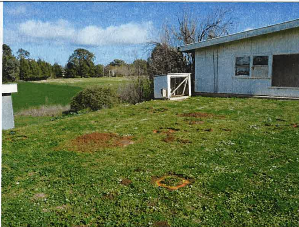
Plate 5 – Soil vapour sampling locations surrounding the underground fuel tanks. Note the two vent pipes on the building.
